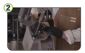
Choose the appropriate blade to obtain the necessary thickness of slices, and secure it into the machine.
