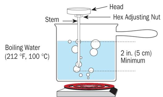
**Note:** The boiling point of water is about 1 °F lower for every 550 feet above sea level. If you are in a high altitude area, the temperature for calibration should be adjusted. For example, if you were at 1,100 feet above sea level, the boiling point of water would be 210 °F.
